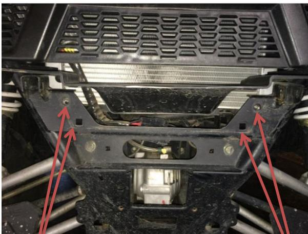
Factory mounting holes to bolt interface
